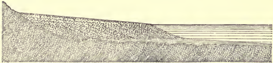
FIG. 32.—Section of a delta, showing inclined beds made in forward growth, with nearly horizontal beds above.—After GILBERT.
